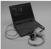
The analog output is controlled by an on-board microprocessor and digital circuitry producing precise drift free signals. The unit is programmed from a PC using Windows® based software and a connection cable. Units may be pre-programmed at the factory or field programmed. All programming information is stored in non-volatile memory in the sensor.
